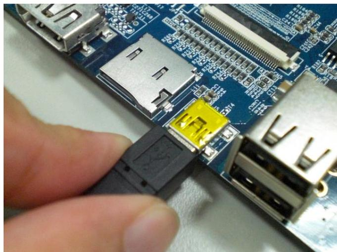
Connect the USB cable to a USB port on the host PC.
