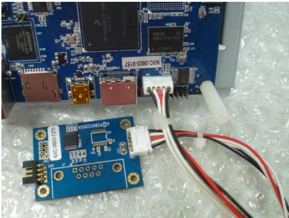
Connect a RS232 IDC cable to C220 debug board
